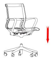
**Step 3**Insert the seat [A] with the armrest into the gas lift [C] with the base [B]. Apply pressure onto seat [A] securing the connection.
