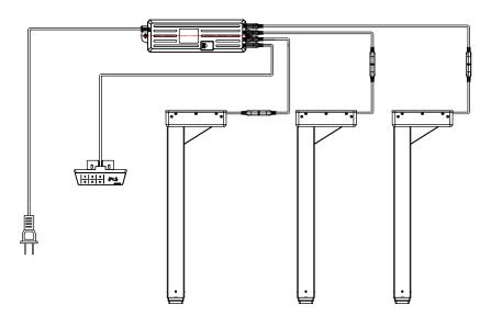
**Step 13:** Install the **H** telescopic cover plates, leaving exit space for the electrical power cords, and secure to worksurface with **N** (8) truss head screws M5\*20mm
