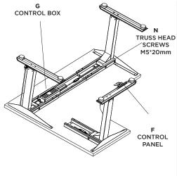
**Step 12:** Connect **F** control panel to **G** control box with **I** connector wires as shown. Use **M** wire manager to secure **I** connector wires to underside of worksurface.
