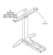
Step 6a: With option of Post foot: Attach O post foot to one column leg with K (4) socket button head bolts, M6\*20mm. Tighten bolts securely. Repeat step 6 with other two legs
