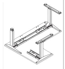
Step 9 & 10: Ensure the leg assembly is still centered, both side-to-side and front-to-back.
