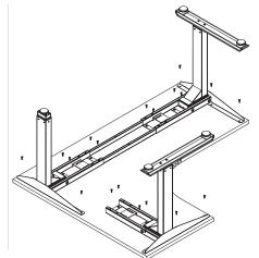
Step 11: Secure the **F** control panel in the desired location with **N** (2) truss head screws M5\*20mm. Insert the **G** control box inbetween crossbeams.
