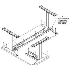
with N 12 truss head screws M5\*20mm.
