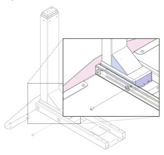
**Step 5:** Remove **C** pad after leg installation, then reuse for assembly of other leg(s) repeating steps 3 & 4. **Remove pad when done.**
