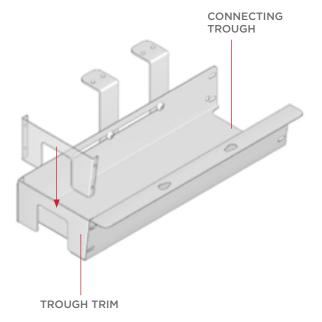
STEP 8. Secure trough trim using (4) self threading screws provided. Trough can now be installed into the Verity structure below the worksurface for Power Infeed to go through trough trim (Refer to Friant Verity Single-Sided manuals for Trough Installation)
