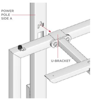
STEP 6B. Inside view of power pole side A mounted onto the U-bracket with (3) M6\*12 screws.
