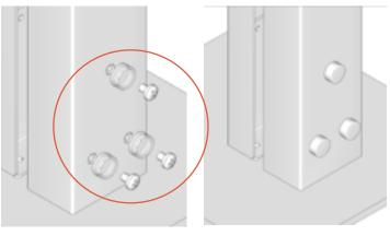
**STEP 6A.** Align power pole side A to the U-bracket. Secure using (3) M6\*12 screws provided.
