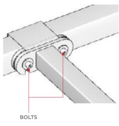
**STEP 3A.** Install power pole base fixed part A onto the base plate using (2) M8\*12 screws provided.
