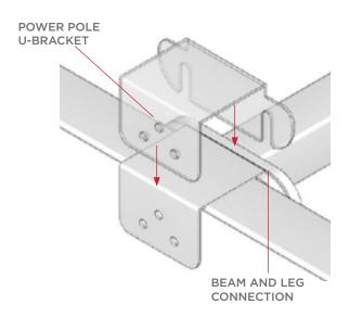
**STEP 2.** Secure bolts to the beam by tightening and applying pressure down onto beam.
