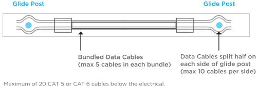
Maximum of 20 CAT 5 or CAT 6 cables below the electrical. Additional cables can be added above electrical if needed
