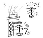
Using the allen wrench, attach the knob to the bottom support using M6x 10mm (2) screws. Place anti-slip rubber on top of the installed knob.
