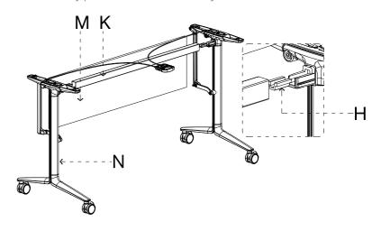
Step 4: Secure modesty panel M to base kit N using (4) wood screws C
