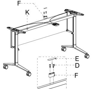
**Step 2:** Attach fixed support bar **K** to base kit **N** using (2) bar supports **H**Position modesty panel **M** within the modesty brackets of base kit **N**
