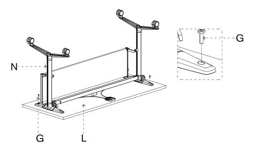
Step 8: Secure the lever to the work top L with (3) wood screws C
