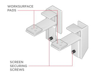
**STEP 3A.** Align the flush brackets on each side of the privacy screen. Insure that they are leveled.
