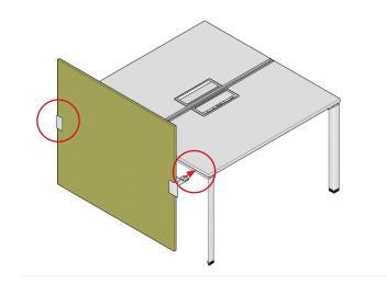
**STEP 6.** Secure privacy screen with brackets to worksurface with (3) screws on each bracket.
