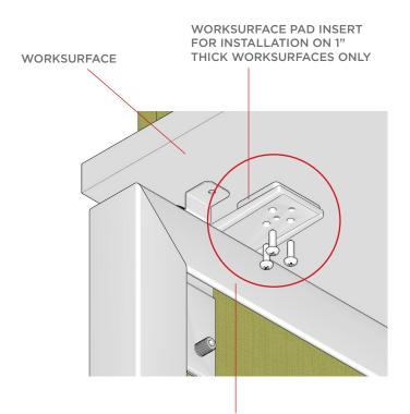
**STEP 7.** Finsihed installation of the privacy screen with flush brackets to a worksurface.
