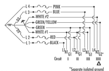
System is rated for connection to a ground 120/240V, 1-PH 60-hz, 20 amp multi-wire branch circuit
