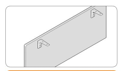
Install brackets (FMOD.BRKT) to Modesty Panel at the pre-drilled holes with the screws provided. The screws go through the bracket into the modesty.
