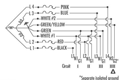
1-PH 60-hz, 20 amp multi-wire branch circuit
