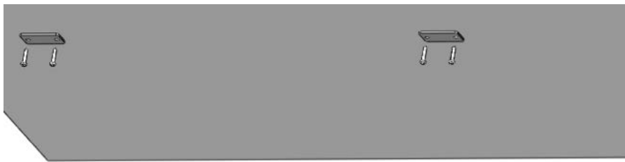
installation of metal plates (for wood overheads only)
